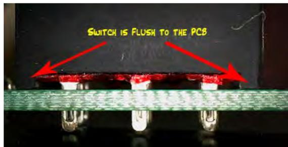
Figure 18 - Footswitch is Flush to PCB
