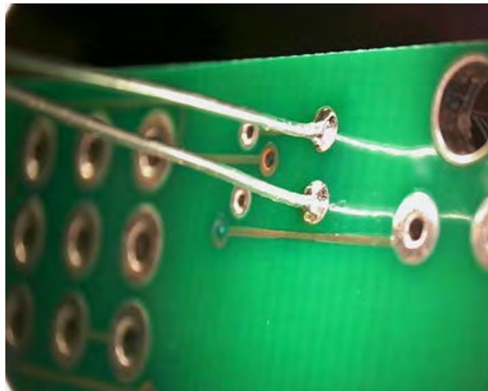
Figure 8 - Nicely Soldered Capacitor Leads
