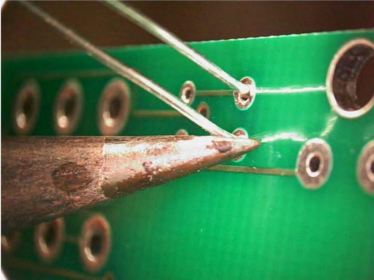
Figure 6 - Hold the Soldering Iron Tip Under the Lead
