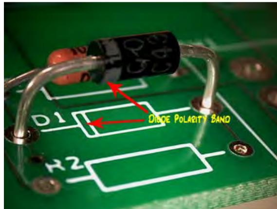
Figure 14 Diode - D1 Polarity Band
