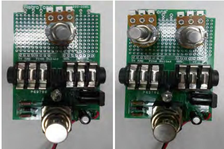
Figure 32 - Potentiometers Mounted on PCB
