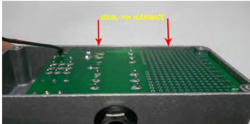
Figure 30 - Level The PCB
