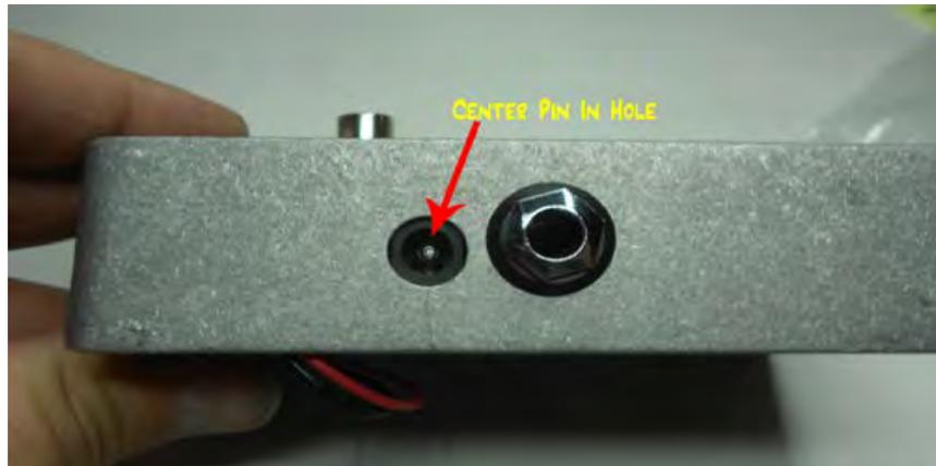
Figure 31 - Center DC Jack Pin In Hole
