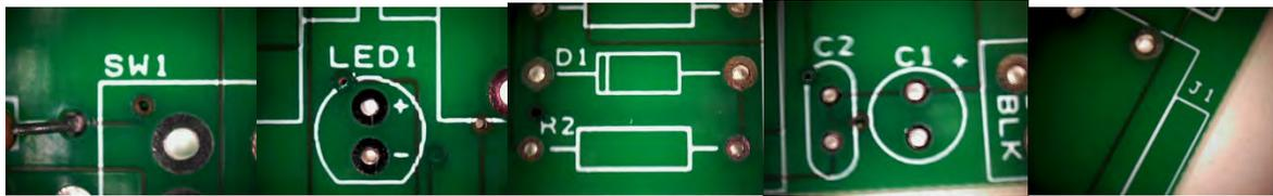
Figure 2 – Example Reference Designators on the PCB
