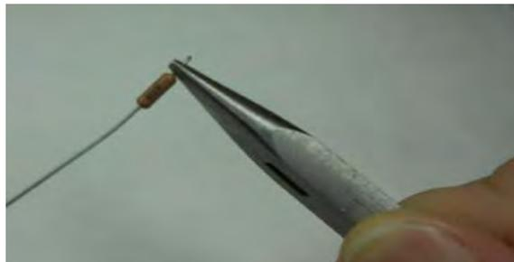
Figure 13 - Bending Axial Leads
