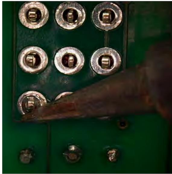
Figure 17 - Heat Up Footswitch Pin
