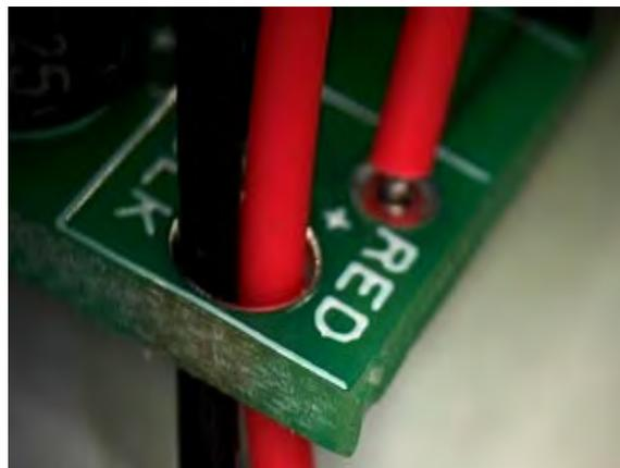
Figure 26 – Battery Snap Strain Relief
