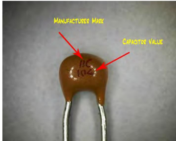
Figure 9 - Ceramic Capacitor Markings
