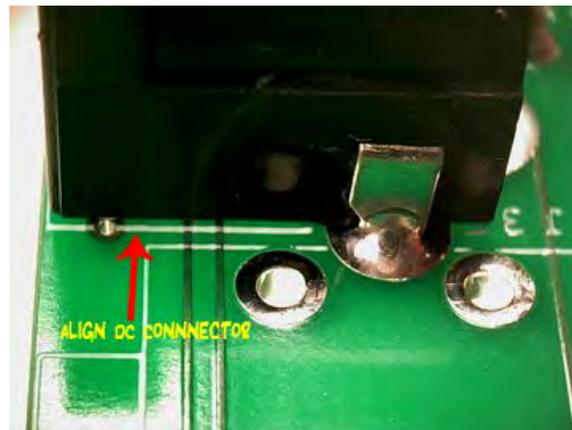
Figure 19 - DC Jack Alignment on Footprint
