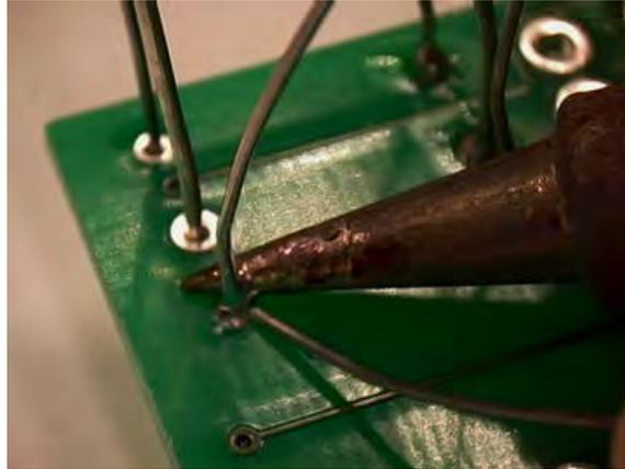
Figure 15 - Soldering Resistor and Diode Leads All At Once
