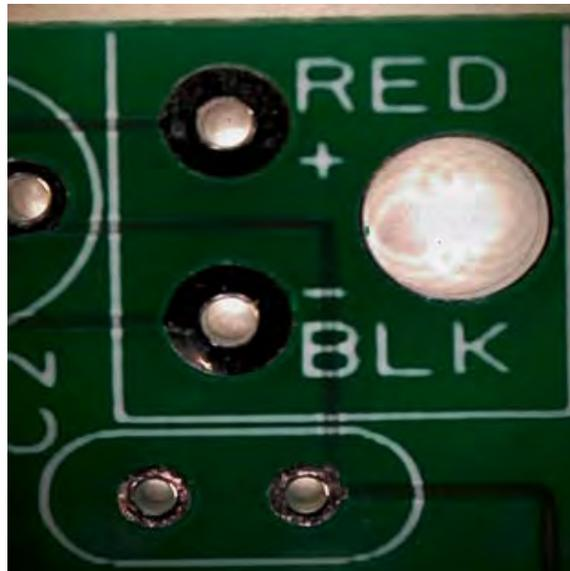
Figure 25 - Battery Snap PCB Footprint
