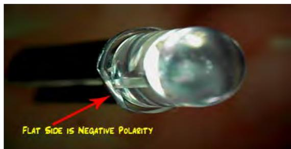
Figure 22 - LED1 Polarity
