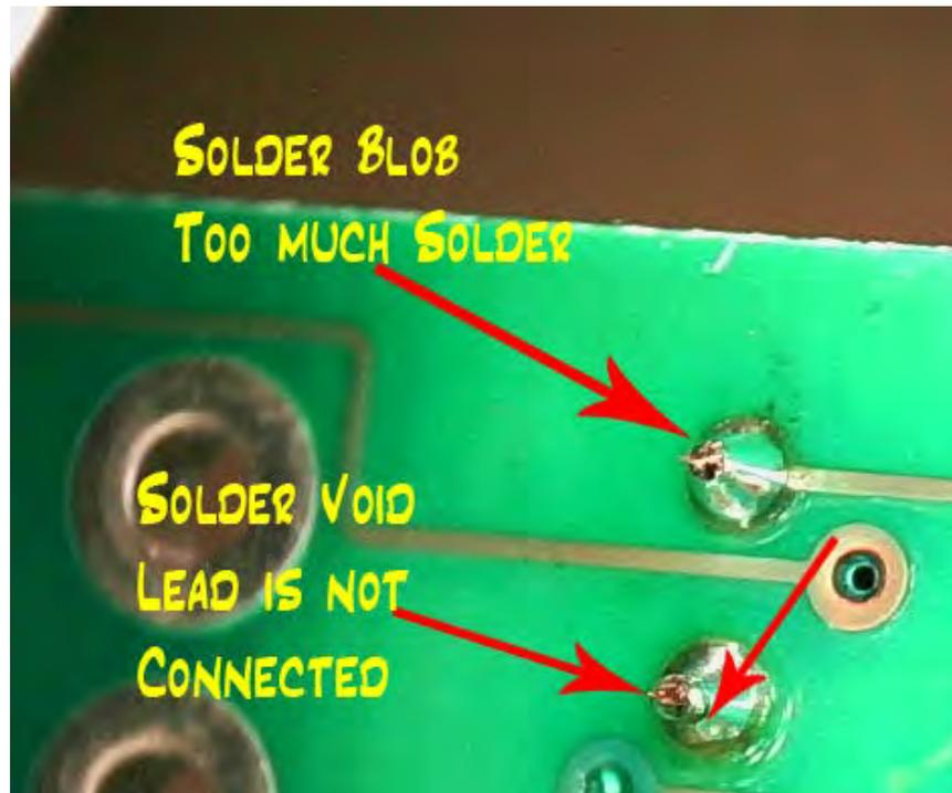
Figure 7 - Two Most Common Soldering Mistakes
