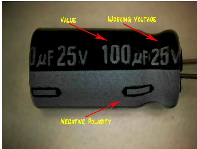
Figure 5 - Characteristics of an Electrolytic Capacitor
