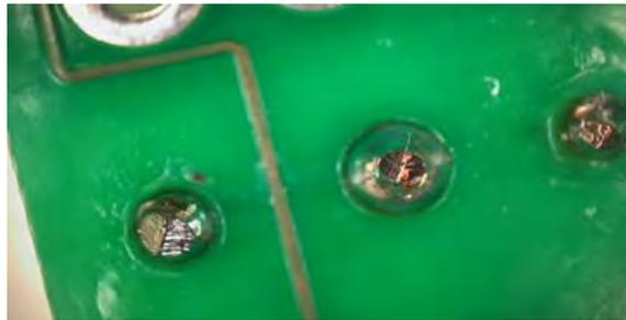
Figure 16 - Cut Leads After Soldering
