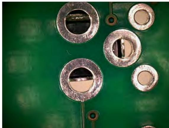
Figure 20 - Large Holes on DC Jack
