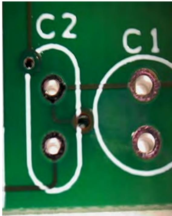
Figure 10 - No Polarity Indication for Capacitor C2
