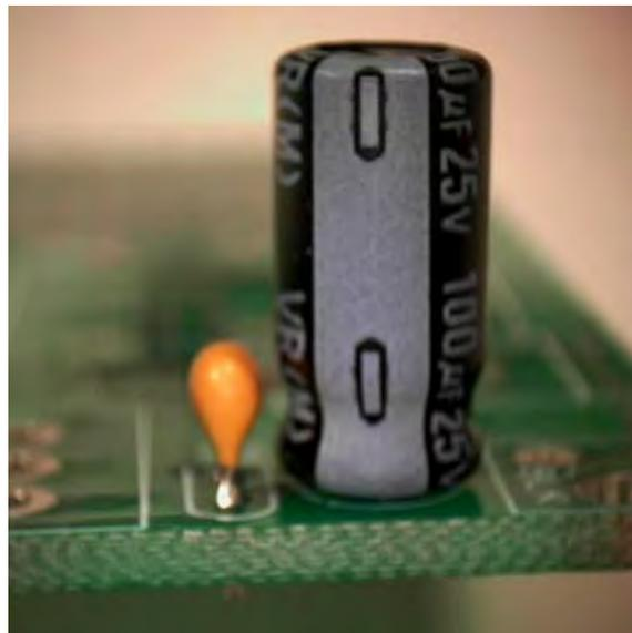
Figure 11 - C1 and C2 Properly fastened to the PCB
