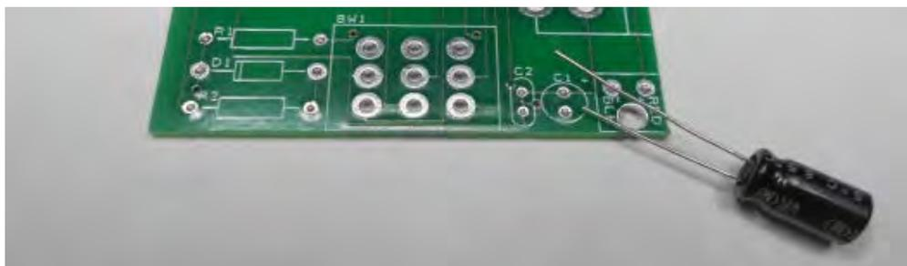
Figure 4 - Electrolytic Capacitor with Long Positive Lead
