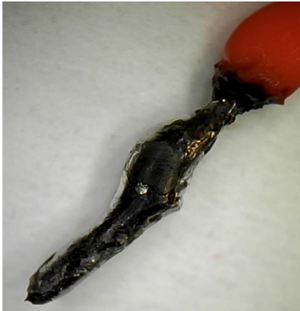
Figure 5 - Too Much Solder
